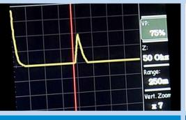
Large, easy to read color display simplifies cable fault locating in most conditions.
