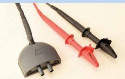
Modules for twisted pair, coaxial and power cables allow the Lexxi T1660 to find cable faults in wide ranging applications, even on live, 3-phase mains cables.
