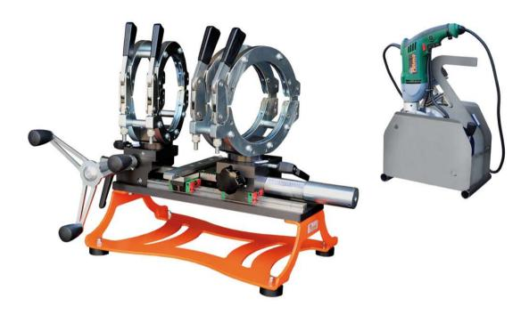
**GAMMA 160** is a manual butt welding machine for HDPE and PP pipes up to Ø 160 mm. GAMMA 160 features special jaws for manufacturing elbows. Machine can also weld moulded fittings like bends, tees, wyes (Y) and flange necks up to Ø160 mm; short flange necks can be welded with the help of a stub end holder (on request), applied to the clamps. Machine body of GAMMA 160 is compact and easy to transport.
