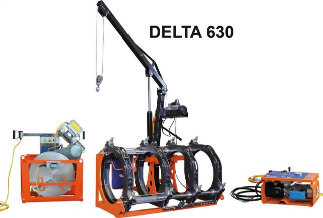
The **DELTA 630** butt fusion machine fuses pipe size from Ø **10" IPS** to **24" IPS** (280 - 630 mm). Designed to serve the large diameter needs of the water, gas and other fluids under high pressure. The machine can weld fittings such as elbows, tees, wyes and flanges. The 1 st and 2nd (movable) and slide along with the pipe. Composed of:
