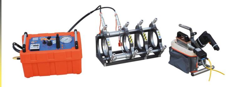
The **DELTA DRAGON 160** hydraulic fusion machines will butt fuse pipe size from Ø 1½" **IPS - 5" IPS** (40 mm - 160 mm). It can butt fuse tees, elbows and other fittings. This is possible because the 3rd clamp can be anchored to the 1 st and 2nd (movable) and slide along with the pipe. Composed of:
