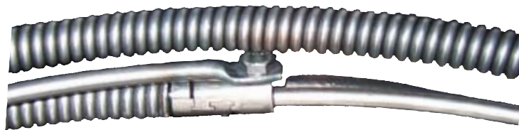
Pictured above is a picture of a CH75-010LW tail piece and A2JK end fitting attached to the inside of a reel.
