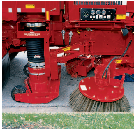
The VacAll features optional heavy-duty, wide area street sweeping with right or left-right side configuration.
